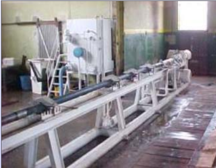
PC Pump test bench
